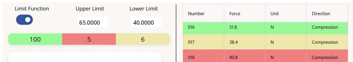
Enable pass and fail highlighting by toggling the Limit Function. Enter the desired upper and lower limit values. Press the “Tab” key or “Enter” key to accept the value.
