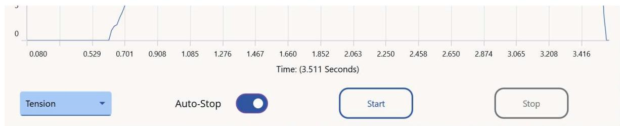
View a live graph of the data while recording a measurement with your force gauge. Select a measurement direction, either tension (pull force) or compression (push force), from the dropdown box. The “Auto-Stop” toggle will automatically stop the recording when zero values are read.
